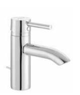
Single lever basin mixer DN 15 ceramic cartridge-K35 cache aerator M 16.5 x 1 1/2" high pressure flexible hose with PEX tubes pop up waste 1 1/4 inch European Standard - EN 817
