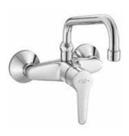
Wall mounted single lever sink mixer DN 15 ceramic cartridge-K35 swivelling (185°) spout I = 200 mm aerator M 22 x 1 flow class A S- unions 1/2 X 3/4 inch European standard - EN 817
