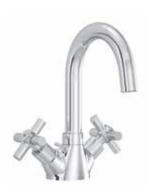
Dual controlled basin mixer DN15 swivel spout aerator M 22 x 1 1/2" high pressure flexible hose with PEX tubes pop up waste 1¼" European Standard - EN 200
