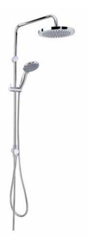
Dual shower system L-shape L = 960 mmwall fastening hand and head shower two way ceramic divertor with 4S hand held shower 1/2 inch ridgeless adjustable shower holder vertically and cylindrically adjustable shower holder shower hose 1/2 x 1/2 inch x 1500mm with fixing kit swivel Round head shower connecting hose mixer to dual shower 1/2 x 1/2 inch x 800 mm
