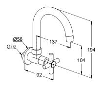
Dual controlled sink mixer DN15 deck mounted with swivel spout aerator M22 x 1 1/2"high presssure flexible hose with PEX tubes European Standard - EN 200
