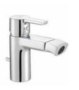
Single lever bidet mixer DN 15 ceramic cartridge-K35 ball joint cache aerator M 18.5 x 1 1/2" high pressure flexible hose with PEX tubes pop up waste 1 1/4 inch European Standard - EN 817
