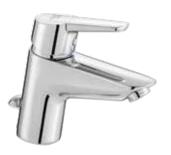
Single lever basin mixer DN 15 ceramic cartridge K-35 aerator M 24 x 1 1/2" high pressure flexible hose with PEX tubes pop up waste 1 1/4 inch European Standard - EN 817
