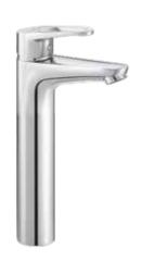
single lever basin mixer XL HR DN 15 ceramic cartridge-K35 aerator M 24 x 1 1/2" high pressure flexible hose with PEX tubes European standard - EN 817
