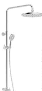
Dual shower system L-shape L = 960 mmwall fastening hand and head shower two way ceramic divertor with 3S hand held shower 1/2 inch ridgeless adjustable shower holder vertically and cylindrically adjustable shower holder shower hose  $1/2 \times 1/2$  inch x 1500mm with fixing kit swivel Round head shower connecting hose mixer to dual shower  $1/2 \times 1/2$  inch x 800 mm
