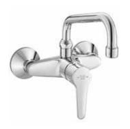
Wall mounted single lever sink mixer DN 15 ceramic cartridge-K35 swivelling (185°) spout I = 200 mm aerator M 22 x 1 flow class A S- unions 1/2 X 3/4 inch European standard - EN 817
