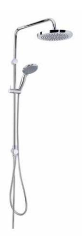
Dual shower system L-shape L = 960 mmwall fastening hand and head shower two way ceramic divertor with 4S hand held shower 1/2 inch ridgeless adjustable shower holder vertically and cylindrically adjustable shower holder shower hose 1/2 x 1/2 inch x 1500mm with fixing kit swivel Round head shower connecting hose mixer to dual shower 1/2 x 1/2 inch x 800 mm
