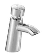
Self Closing Tap - Push type DN 15 push type cache type aerator M16.5x1 minimum working pressure 0.1bar maximum working pressure 3 bar time of water flow 0 to 16sec with 2mm allen key for time adjustment
